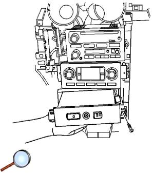
3. Install the communication interface module screws.
