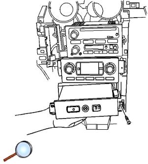
2. Remove the screws that hold the communication interface module to the I/P.
